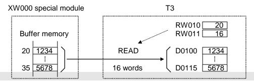
Note 1) The special module can be designated not only by the assigned register, but also by the mounting position. The mounting position is designated by a constant data for the operand A as follows.
